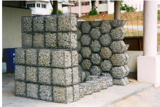
Figure 3. Various Gabion Configurations Developed for Experimental Testing (Ramli et al., 2013)
